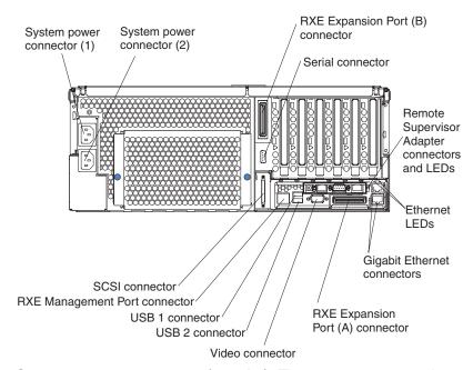
**System power connectors (1 and 2):** The system power cords are connected to these two connectors to provide power to the system.
